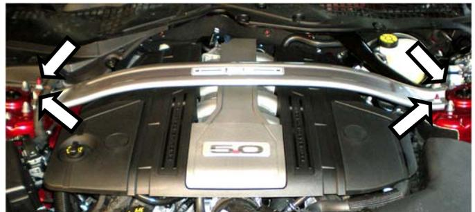
2. Remove the stock engine cover. Using a small flat blade screw driver, carefully remove the (2) round covers located at the front right & left of the engine cover. Using a 10mm socket, remove the retaining nuts from both locations. Remove the cover and set aside, with the nuts, in a safe location for reinstallation.
