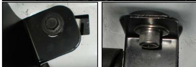
8. Using a 10mm socket, remove the coolant reservoir from the stock location. Install the relocation bracket supplied with our kit using the stock fasteners. Reinstall the stock reservoir on the new bracket using the fasteners supplied. Use a 3/16" allen wrench and 7/16" box wrench to tighten.
