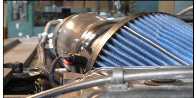
15. Reinstall the stock intake cover using the stock nuts and 10mm socket. Reinstall the round covers to finish the install.
