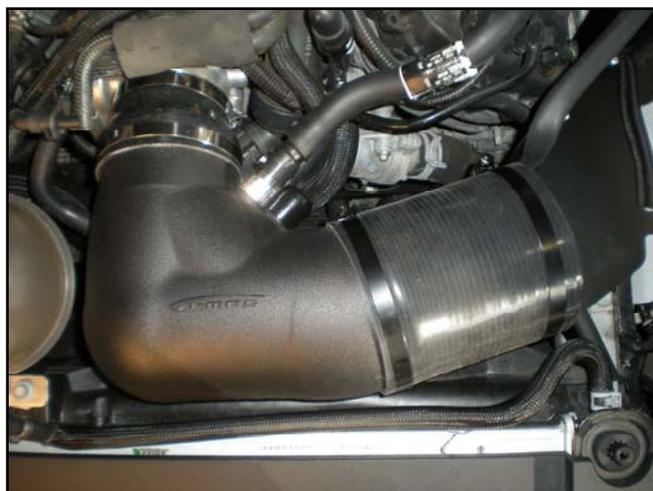
10. Using an 11/32" wrench and lock nuts supplied, install the cone air filter on the PMAS MAF housing (**DO NOT OVER TIGHTEN**). Using the #6-32 self tapping screws supplied, install the MAF sensor.
