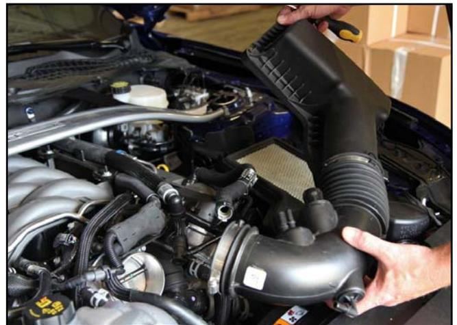
5. Using a 10mm socket, remove the single mount bolt from the lower air cleaner housing. This is located to the right of the housing on the fender well. Retain this fastener for the PMAS installation. Remove the housing from the engine bay and set aside.
