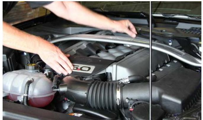
2. Unplug the Mass Air Flow sensor. This is located in the air cleaner lid tube. Pull back on the red tab located at the back of the connector to unlock it (see photo). Once unlocked, unplug the connector from the sensor.
