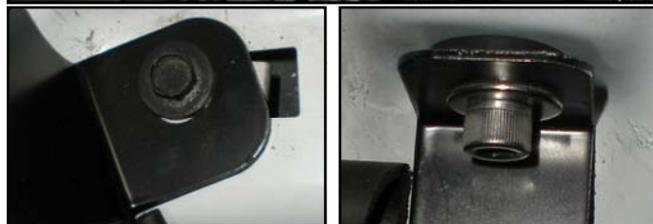
7. Using a 10mm socket, remove the coolant reservoir from the stock location. Install the relocation bracket supplied with our kit using the stock fasteners. Reinstall the stock reservoir on the new bracket using the fasteners supplied. Use a 3/16" allen wrench and 7/16" box wrench to tighten.
