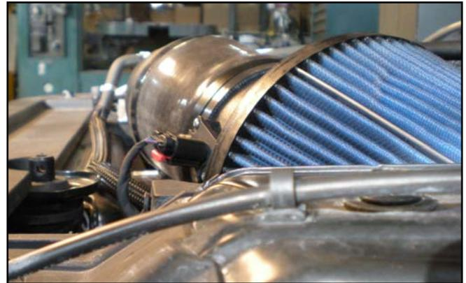
14. Reinstall the stock intake cover. Align the cover with the clips on top of the intake and push down firmly.
