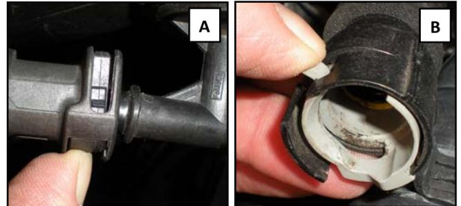
4. Loosen the hose clamp at throttle body inlet and release the retainer clips for the air cleaner lid. Remove the intake tube/air cleaner lid assembly from the engine bay and set aside.
