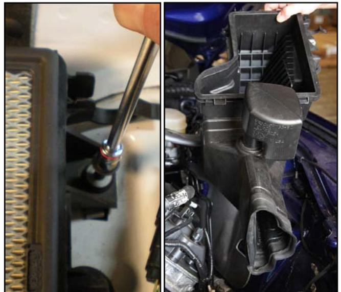
6. Install the PMAS heat shield in the stock air cleaner housing location. Align the upper mount tab with the stock mount location and install the stock mount bolt retained from housing removal, **DO NOT TIGHTEN**. Push the rubber Wellnut into the hole in the inner fender well. Once it's fully seated against the fender well, use a 3/16" allen wrench to tighten the socket head screw securely. Using a 10mm socket, tighten the stock mount bolt.
